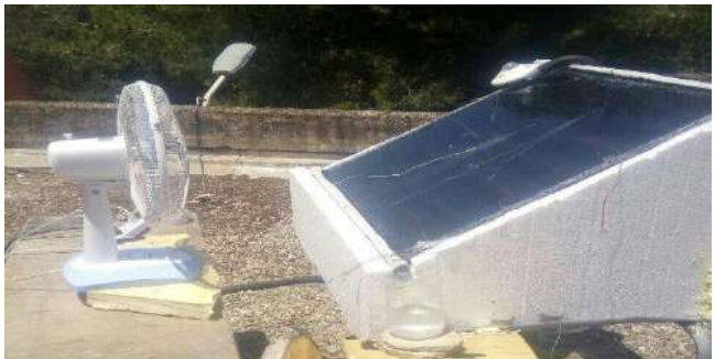
Fig.2. Cooling the outside of surface
